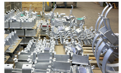
Galvanized pipe bearings in a wide range of designs for shipping in accordance with customer guidelines
